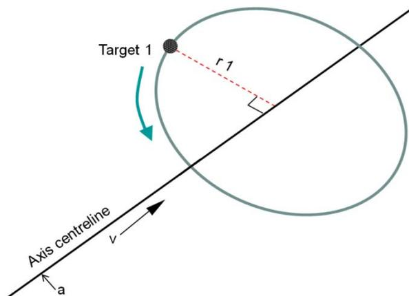
Figure 2. Rotation of a target about an axis.
