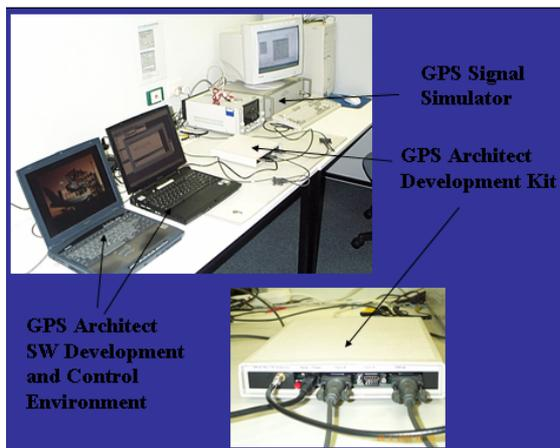
Fig 9 GPS testing and simulation environment
