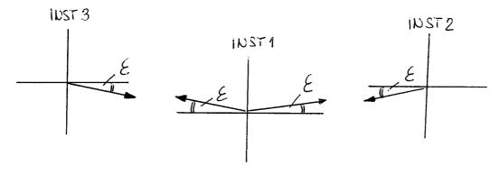
Adjust level  $J_4$  to  $J_3$  and check with  $J_2$  (or  $J_1$ ). (Adjust level  $J_5$  to  $J_1$  and check with  $J_2$  (or  $J_3$ ).
