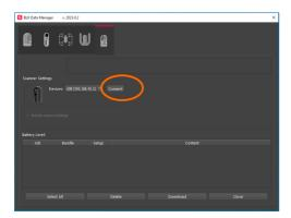
Turn on BLK360 and plug USB-C / USB-A cable to connect to computer. Click Connect.
