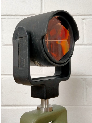
Leica / Wild GPH1 + GRP1 circular prism
